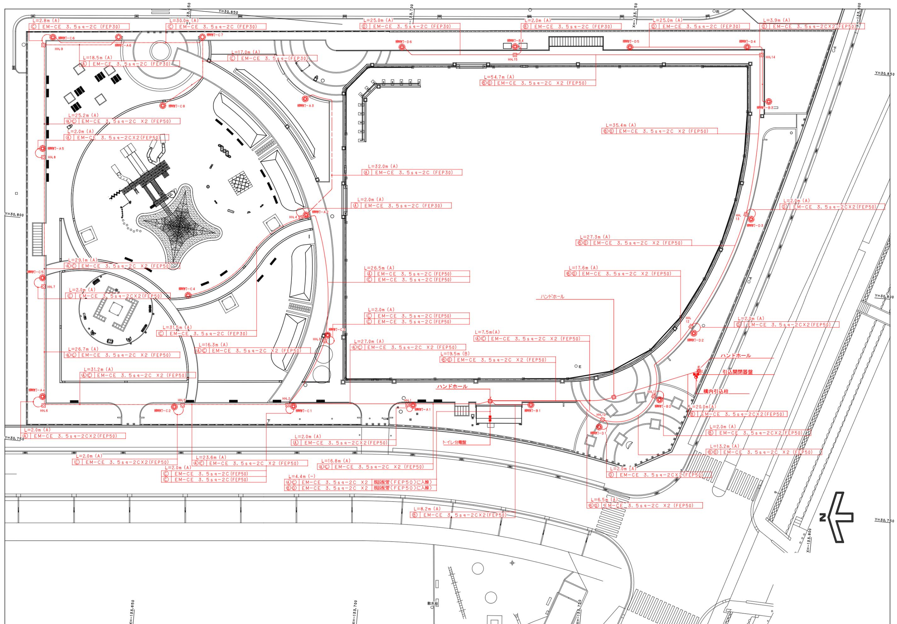
L=2.8m (A) (C) EM-CE 3.5sq-2C (FEP30) L=30.0m (A) (C) EM-CE 3.5sq-2C (FEP30) L=25.0m (A) (D) EM-CE 3.5sq-2C (FEP30) L=2.0m (A) (B) EM-CE 3.5sq-2C (FEP30) L=25.0m (A) (D) EM-CE 3.5sq-2C (FEP30) L=3.9m (A) (D) EM-CE 3.5sq-2CX2 (FEP50)
